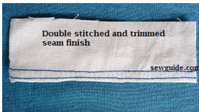
Figure 4.1 trimmed seam finish
